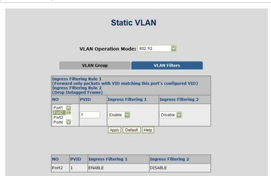
Figure 53: 802.1Q Ingress filter interface
